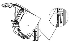
Use the holder at the back of the unit against on the mounting plate to prop up the unit
