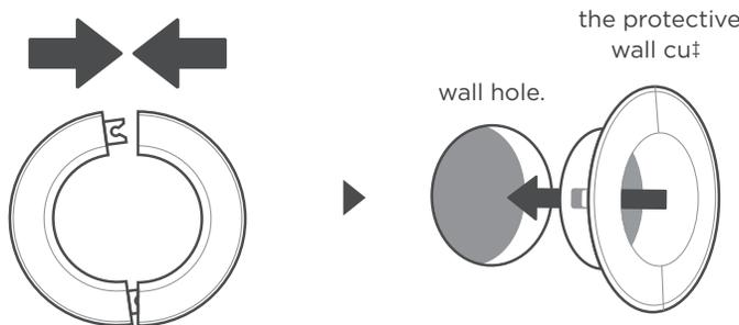
Place the protective wall cut in the hole .
