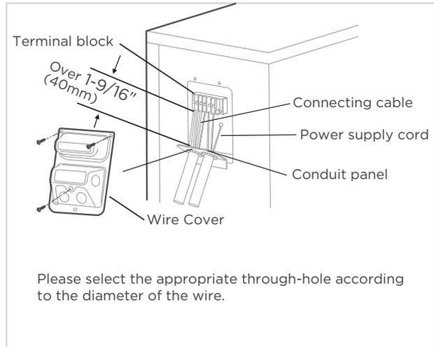
**How to properly connect the wire lines.**
