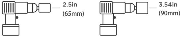
Using a 2.5in(65mm) or 3.54in(90mm) core drill(according to the unit you purchased )
