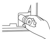
To prevent unwanted leaks you must plug the unused drain hole with the rubber plug provided.
