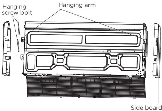
9. Mount the indoor unit onto the hanging screw bolts with a block. Position the indoor unit on a flat level by using a level to prevent leaks.
