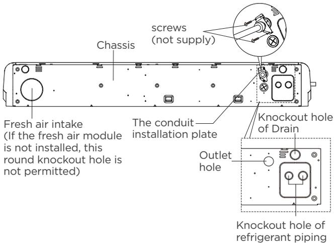
**NOTE:** When installing, open the corresponding round knockout holes as shown in the illustration, rectangular knockout holes are not permitted.
