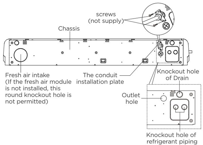
**NOTE:** When installing, open the corre sponding round knockout holes as shown in the illustration, rectangular knockout holes are not permitted.
