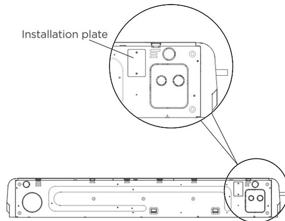
2. The installation plate is used to block the outlet holes at the bottom of the base when out of the side line.
