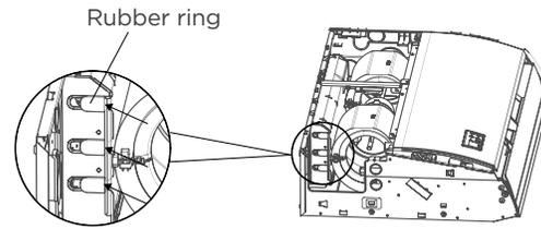
1. Rubber rings are used to block the excess space in the three crossing holes of the electronic control box.
