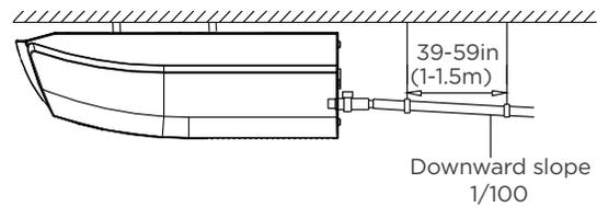
1. Cover the drainpipe with heat insulation to prevent condensation and leakage.
