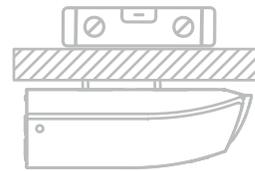
The ceiling is horizontal and its structure can sustain the weight of the indoor unit.
