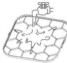
If using water, the inlet side should face down and away from the water stream.
