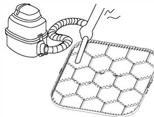
If using a vacuum cleaner, the inlet side should face the vacuum.
