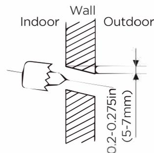
**NOTE:** When the gas side connective pipe is  $\Phi$  5/8in (16mm) or more, the wall hole should be 3.54in (90mm).
