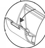
Before fixing this screw, you need to open the screw cover; and after fixing screw, please close the cover.
