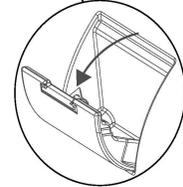
Before fixing this screw, you need to open the screw cover; and after fixing screw, please close the cover.
