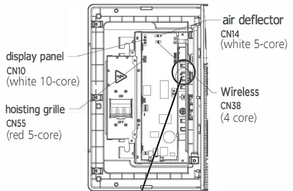
when connection is completed, please clip the wires to the buckle.
