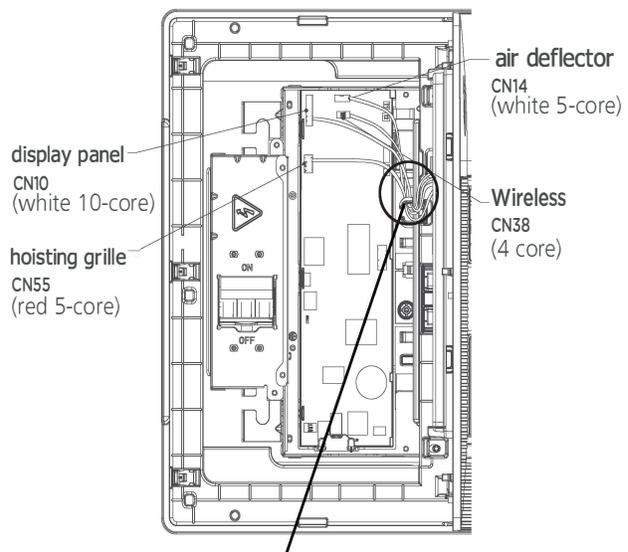
when connection is completed, please clip the wires to the buckle.
