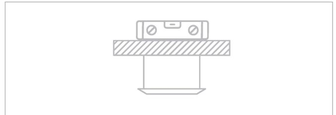
The ceiling is horizontal and its structure can sustain the weight of the indoor unit.
