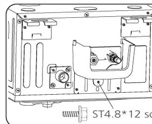
**NOTE:** Two ST4.8\*12 screws are supplied, one of which is spare.
