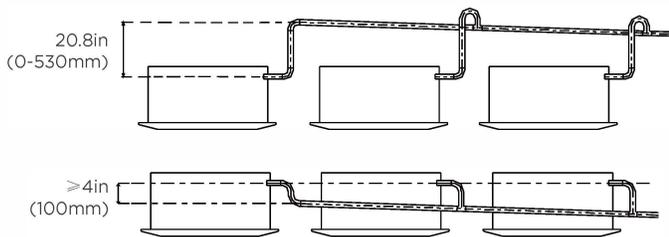
Pass the drain hose through the wall hole. Make sure the water drains to a safe location where it will not cause water damage or a slipping hazard.
