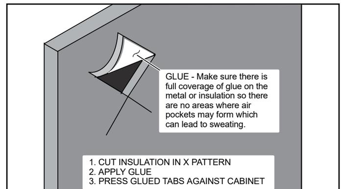
Figure 12. Repairing Insulation
