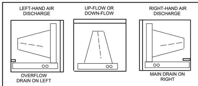
**Figure 8. Main and Overflow Drain Locations Based on Coil Orientation**
