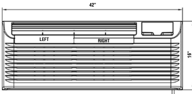
AIR DISCHARGE GRILLE IS REVERSIBLE TO PROVIDE EITHER 55° OR 15° DISCHARGE ANGLE
